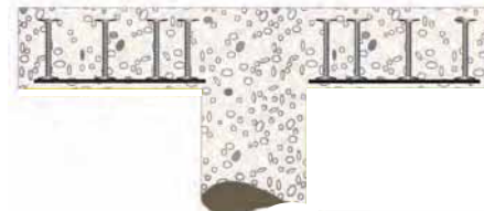
DSA Reinforced Column
